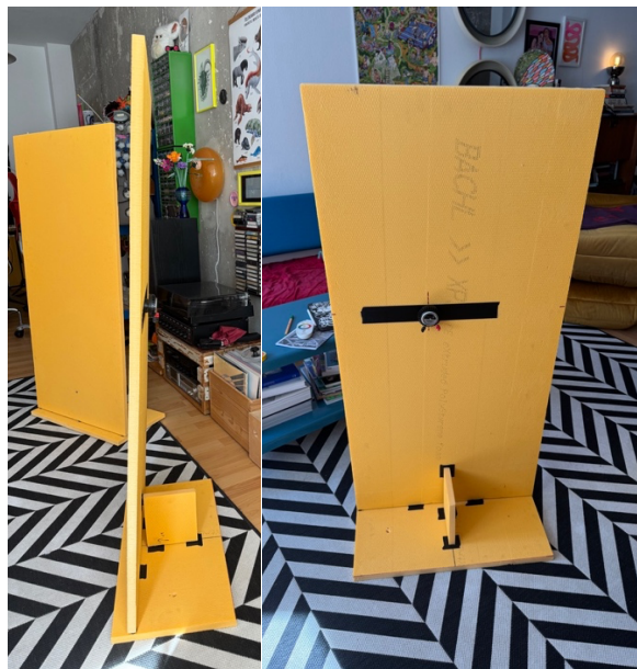
Figure 23: Custom speaker design from Styrodur 3035 CS panels and the Dayton Audio DAEX32EP-4 exciter
