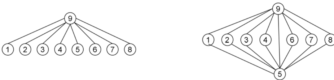
Figure 2: Clear interactions graphs for designs 9-4.1 (left) and 9-4.2 (right) Vertices are labeled with factor numbers (cf. Table 1 in the appendix for corresponding Yates matrix column numbers).
