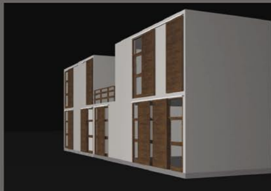
fasade composition an sunprotection through shiftable elements
