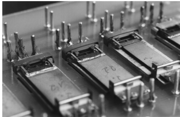
Fig. 12 Mini series of piezo relays as a prototype with device data: length \approx 20 mm, width \approx 9 mm and height \approx 2 mm
